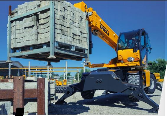
Better than a conventional telehandler: continuous turret rotation provides full operational coverage with a single positioning.
