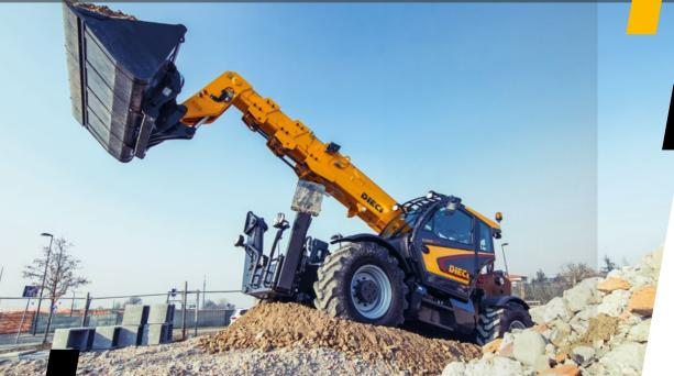
Icarus, in the New Construction Range, is the vehicle that reaches great heights: it can extend **up to 18 meters**, guaranteeing **maximum stability** thanks to the independent outriggers.
